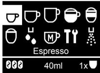
The selected speciality coffee is shown on the display screen by a symbol, e.g., an espresso cup, and in clear text, e.g., “Espresso”.
